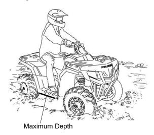
Your ATV can operate through water with a maximum recommended depth equal to the bottom of the footrests. Follow these procedures when operating through water:
